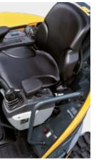
In a 9A series cabin, you can easily adjust the seat and wrist rests settings to best suit your preferred operating condition. The left and right control levers are ergonomically located for convenient access. A safety lock system is designed to prevent exiting the cabin while hydraulic controls are live. When the safety lever and left side console are positioned upright, hydraulic functions are disengaged.
