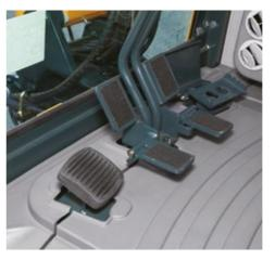
Pedals All pedals are foldable for additional floor space. Footrest, attachment pedal, left and right travel pedals and boom swing pedal are arranged for convenient access.
