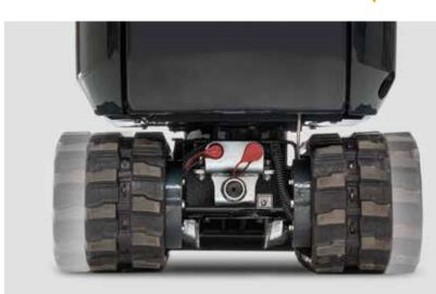
Hydraulic hammer piping is integrated as standard for efficient hammer operation inside buildings.
