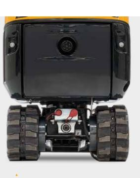
An external hydraulic oil tank keeps oil cooler without an additional cooling system. This protects performance in high ambient temperature.
