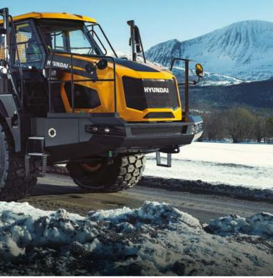
The optional heated body prevents frozen material sticking to it, enabling quicker and
