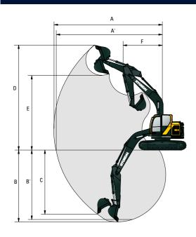
**Boom Length** 5,680 (18' 8") 2,400 (7" 10") 2,920 (9' 7") 9,040 (29' 8") 9,430 (30' 11") 9,910 (32' 6") A Max. digging reach Max. digging reach on 9,750 (32' 0") 8.860 (29' 1") 9,260 (30' 5") Max. digging depth 5,750 (18' 10") 6,150 (20' 2") 6,670 (21' 11") 6,490 (21' 4") Max. vertical wall 5,120 (16' 10") 5,570 (18' 3") 6,090 (20' 0") digging depth Max. digging height 10,820 (35' 6") 7,900 (25' 11")
