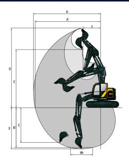
Unit: mm (ft·in) **Boom Length** 5,650 (18' 6") 2-Piece A | Max. digging reach 9,050 (29' 8") 9,460 (31' 0") 10,020 (32' 10") Max. digging reach on 9,860 (32' 4") 8,880 (29' 2") 9,290 (30' 6") Max. digging depth 5,460 (17' 11") 5,860 (19' 3") 6,380 (20' 11") 5,750 (18' 10") 6,270 (20' 7") Max. vertical wall 4,530 (14' 10") 4,970 (16' 4") 5,520 (18' 1") digging depth Max. digging height 11,470 (37' 8") 8,540 (28' 0") Min. swing radius 2,000 (6' 7")
