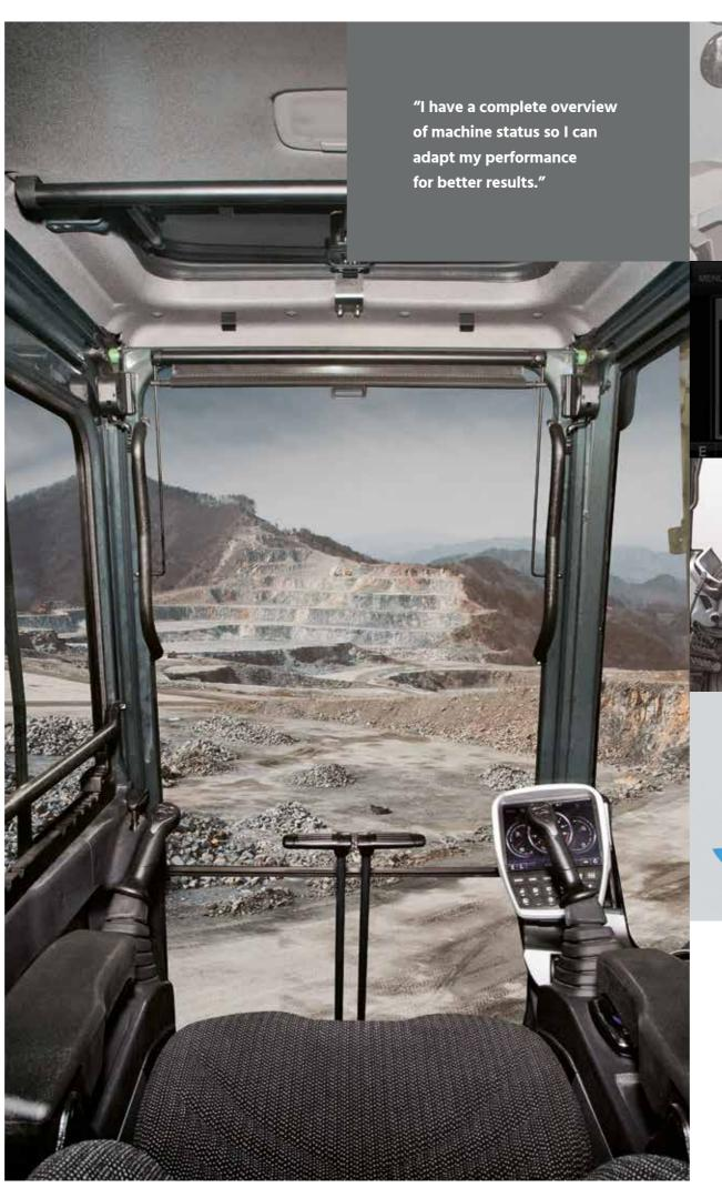
The instrument panel is optimised to provide quick, easy access to machine status information as you work. It features an 8-inch touchscreen monitor for excellent legibility.
